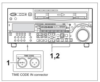
**1** • When synchronizing to an external time code output (LTC):
